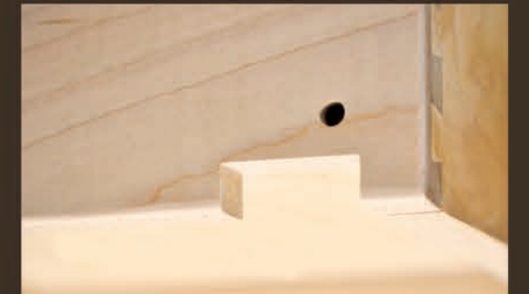
Notch and Drill for Self-Closing Undermount Slides
